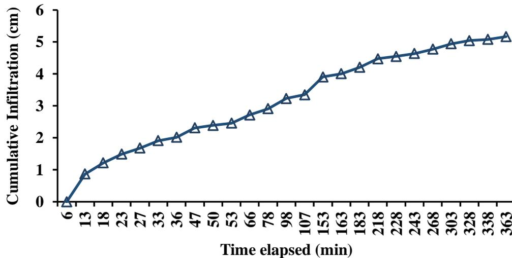
**Figure 6.** Cumulative infiltration into 2m furrow length and average furrow width. The X-axis represents the time elapsed in minutes while Y- axis represents the cumulative infiltration in cm into 2m furrow length and average furrow width.
