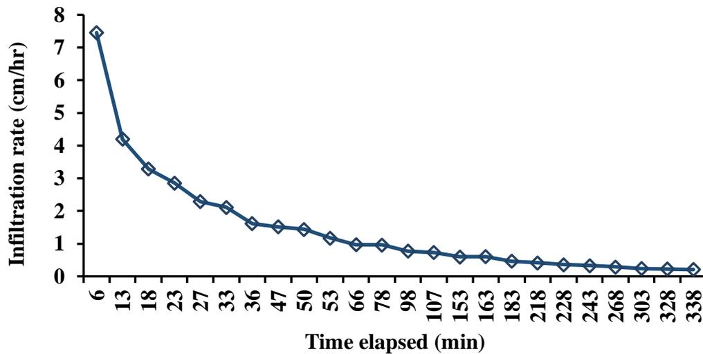
**Figure 4.** The soil infiltration rate for 2 m furrow length is shown where the X-axis represents the time elapsed in minutes while Y- axis represents the infiltration rate in cm/hr per 2 m furrow length and average furrow width.
