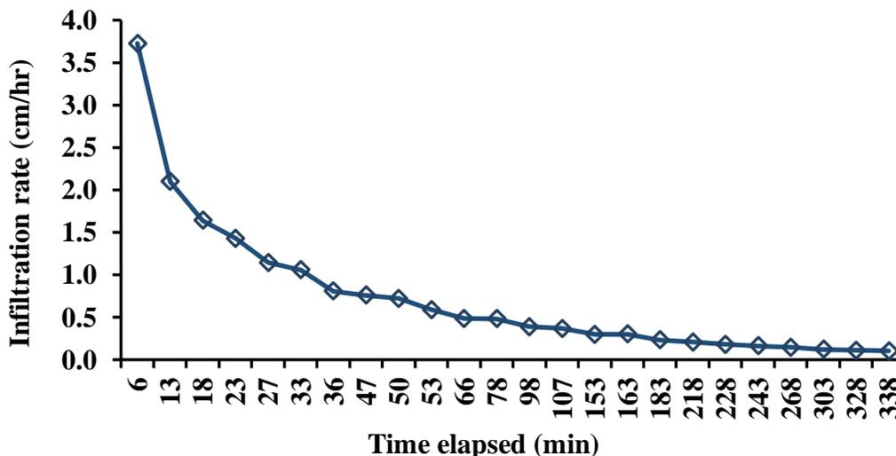
**Figure 3.** The soil infiltration rate plotted with time elapsed showed a greater infiltration rate when the experiment commenced and then dropped gradually till the end of the experiment as displayed. The X-axis represents the time elapsed in minutes while Y- axis represents the Soil infiltration rate in cm/hr per 1 m furrow length and average furrow width.
