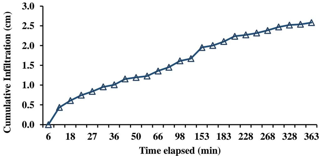
**Figure 5.** The cumulative infiltration of 1 m furrow length and furrow width area in cm plotted against time. The X-axis represents the time elapsed in minutes while Y- axis represents the cumulative infiltration in cm into 1 m furrow length and furrow width.
