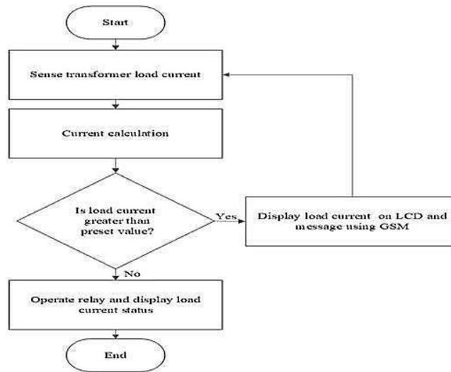
Figure 2 Flowchart for transformer load conditions
