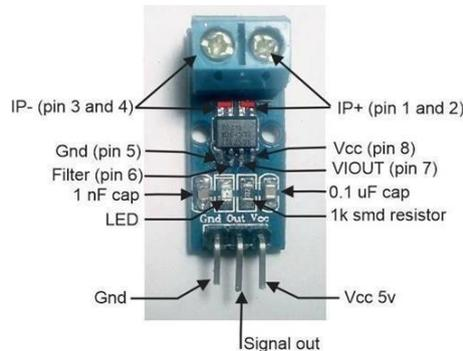
**Figure 5 Current sensor (ACS712-20A module)**
