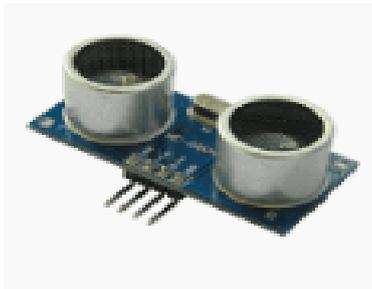
The Ultrasonic Sensor integrated with Arduino is used for sewage overflow detection. This will continuously monitor the sewage level so that the overflow can be prevented in advance.
