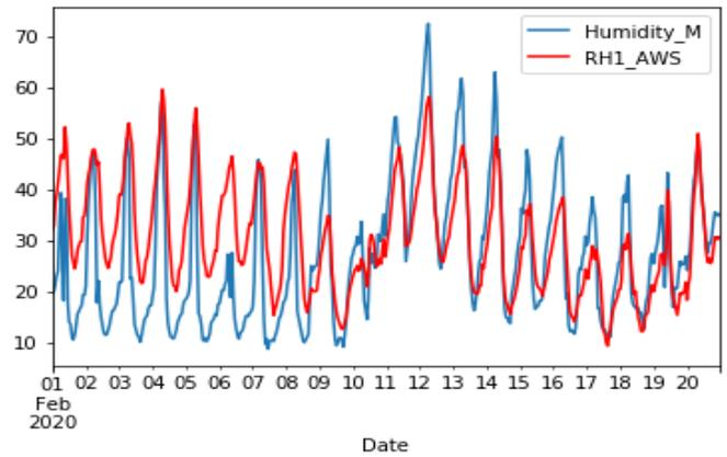
Figure 4(b) Humidity comparison to All Weather Station
